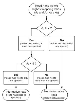
**Figure 2.** Flow diagram of the  $\gamma$ - $\delta$  algorithm. Only the two highest mapping ratios to two reference genomes of a single read are required. In the figure, it is assumed that the highest mapped ratio  $A_i$  belongs to the reference genome *i*.
