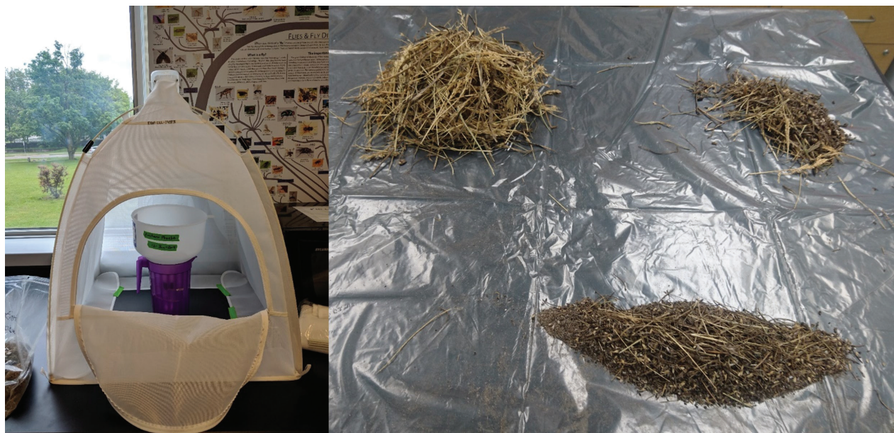
Figure 1. Emergence trap with Berlese-Tullgren funnel (left picture) and nest separated into components >5 mm, >2 mm and <2 mm via consecutive sieving. Individually removed arthropod remains are not displayed.
